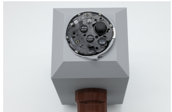
(f) Finally, we embed the main tracking electronics after attaching the ribbon cable. At last, the black cap needs to be added. The final result is shown in Figure 1(c).
