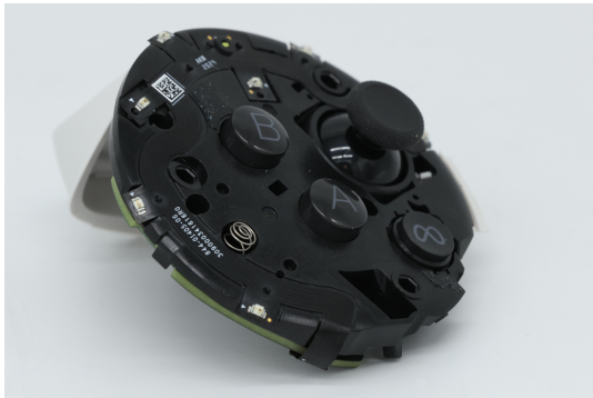
(c) The main tracking board contains the buttons and IR LEDs for tracking. It should be placed in the fabricated object so that the cameras of the Quest HMD can see the LEDs.
