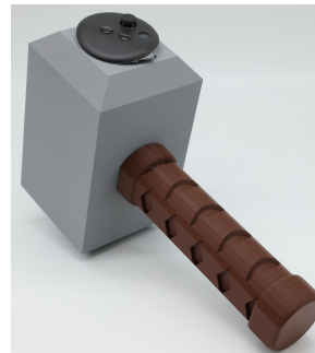
(c) A 3D-fabricated medieval fantasy hammer that allows for embedding the controller's tracking electronics into its hammer head.
