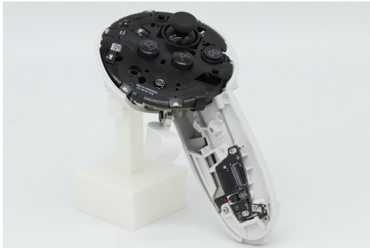
(a) First, the screws need to be removed that are located in the battery compartment below the sticker, to remove one half of the casing.
