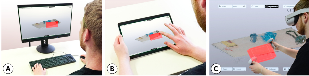
Figure 5. Study conditions to compare point cloud segmentation on a desktop PC (A), a tablet (B), and virtual reality (C) regarding their suitability for segmenting simple and complex point clouds. All pictures display the training scene of the study containing the Utah teapot as the target object.
