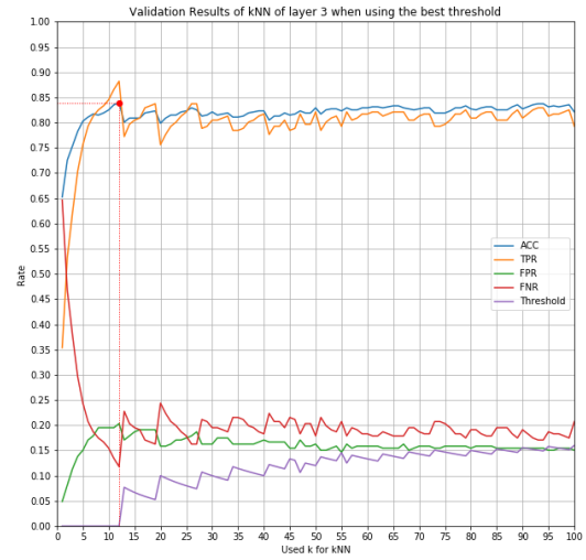
Figure 10: Determination of the best value for k and the corresponding best threshold for layer 3. For every k , the corresponding threshold meeting the EER is calculated. The validation results show that the highest accuracy can be achieved using k = 12 for layer 3 (red dashed line).
