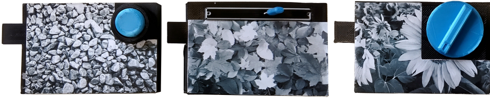
Fig. 4. Three example modules developed as an initial set for the ARm Haptics system. Left: button module (binary input: pressed, not pressed). Center: slider module (discrete input: 100 levels). Right: knob module (discrete input: 100 levels).
