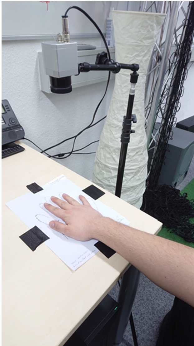
Figure 4: The setup of the controlled study, which was used for data collection. The camera was mounted on a height of 37 cm.
